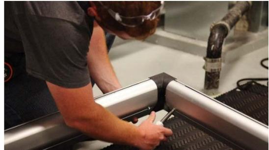
Locate pre-drilled mounting holes on Sensor Flow Frame. Match the NJK Sensor Module to the mounting holes in the Sensor Flow Frame and secure the Sensor Module to the sensor frame by four screws (Included).
