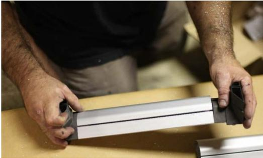
Slide extrusion side piece onto sensor bottom piece corner (set screws in corner pieces may need to be loosened to allow the side piece to slide into place). Tighten set screws snugly to extrusion piece. Repeat for other side piece.
